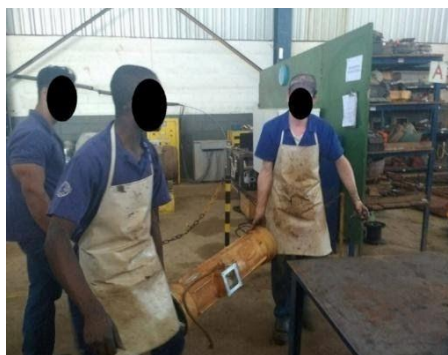
Figure 1 - Manual loading of engines in pairs
