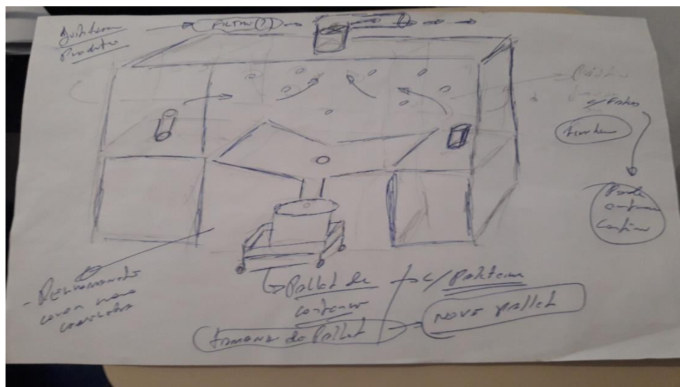
Figure 11. Sketch of chemical waste hood
