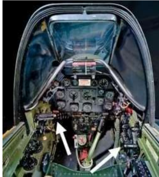
Figure 2 - Cockpit of a P-51D. The arrows show the throttle (left) and hood opening handle (right)
